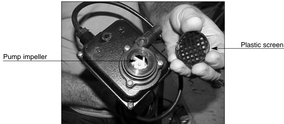
Figure WC-1HP.06 - Pump
