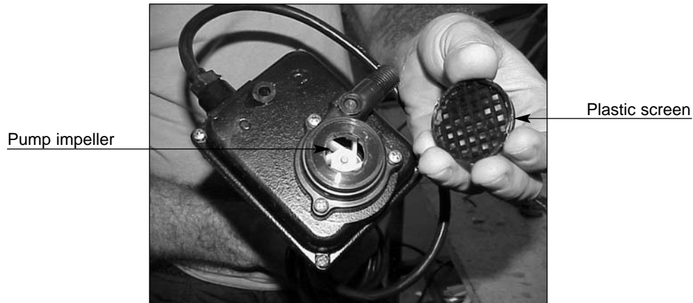
Figure WC-1HP.06 - Pump
